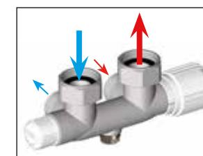
In order to change the valve configuration from single-pipe to double-pipe, close the by-pass screw. When the valve is in double-pipe configuration, it must be installed with the water connection always placed on the thermostatic valve side, in order to avoid noisiness in case of automatic operation (by using a thermostatic head).
