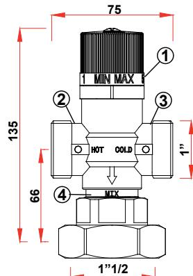
If the thermostatic mixer is installed on a fix point regulating unit for under floor heating system, the temperature value is readable on the thermometers of the unit. Once fixed the handle position of the mixer, the system is regulated.
