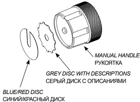
If required the installation of electric heads, unscrew the manual handle and screw the electric actuator.
