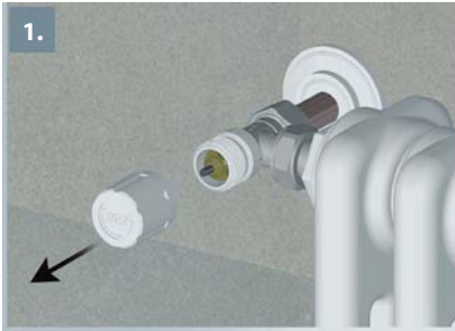
1. Unscrew the manual regulating valve
