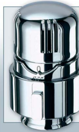
Art. 1827 Chrome-plated thermostatic head. Built-in sensor with liquid-filled element. - Temperature range: from 7°C to 28°C
